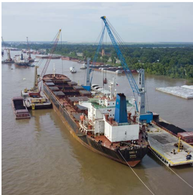
St. James Stevedoring is an Example of a Coal Port in the Gulf of Mexico that Employs Highly-Efficient Midstream Loading of Coal onto Ocean Going Vessels
