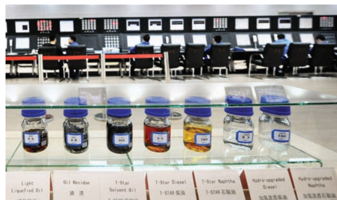
The two samples on the right are the end products of the DCL process.
