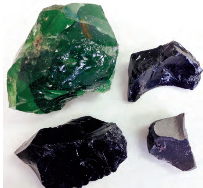
Slag captured from the gasification process (photo provided by Westinghouse Plasma Corp., a division of Alter NRG)
